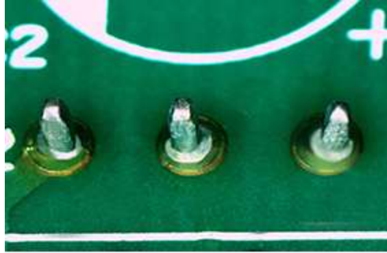
Example of soldering on substrate
